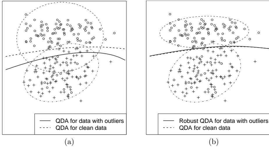
Figure 11: Two groups of data simulated from bivariate normal distributions with different means and covariances. 10% of the data points from the first group ( $\circ$ ) were sampled from the distribution of the second group ( $+$ ). QDA separation curves are shown when using classical parameter estimates (a) and robust MCD estimates (b).
